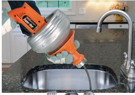
Switch to a different diameter cable with the Quick-Change Cable Cartridge. You just loosen three screws, pull the front of the drum off the cable, and load in another cartridge. Changing takes less than a minute and turns what could be a messy job into a clean one.
